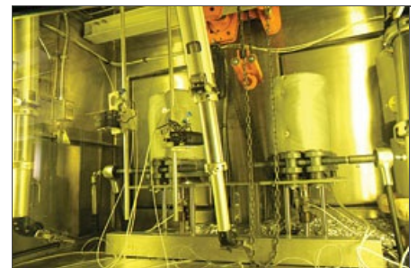
The new Irradiation-Assisted Stress Corrosion Cracking (IASCC) test rig at INL's Materials and Fuels Complex is a unique facility that can inspect highly radioactive materials.
